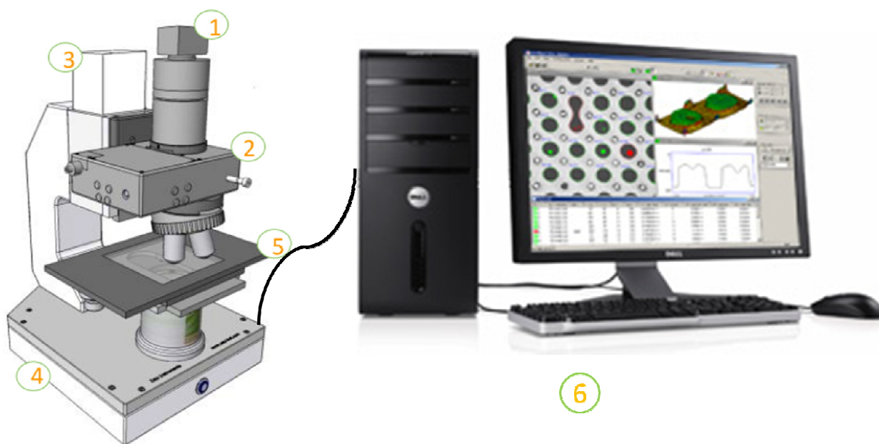
Figure 2. Schematic view of the Zeta 20 3D system
