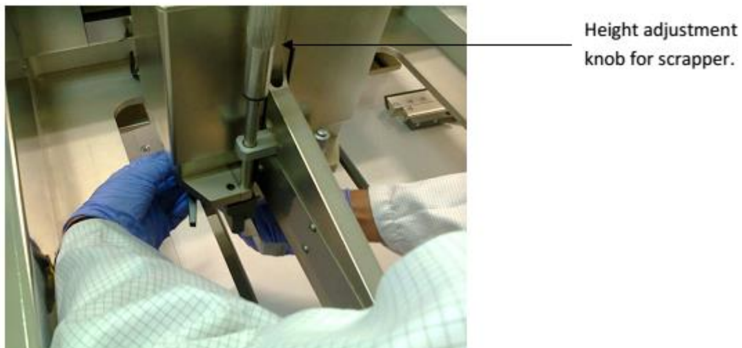
Figure 11. Micro-height adjustment knob for scraper
