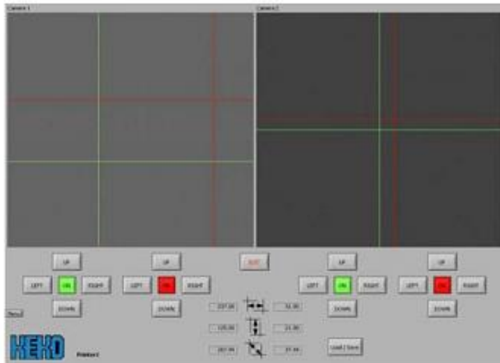
Figure 17. Cross-hair view of cameras with the two set of cursors for respective views
