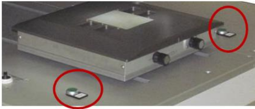
Figure 15. Mechanical 'PRINT' buttons on either side of the vacuum chuck
