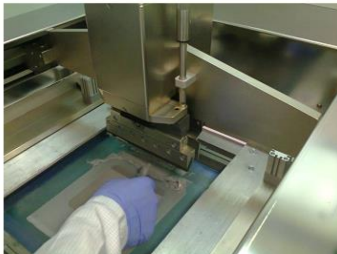
Figure13. Paste application on the screen
