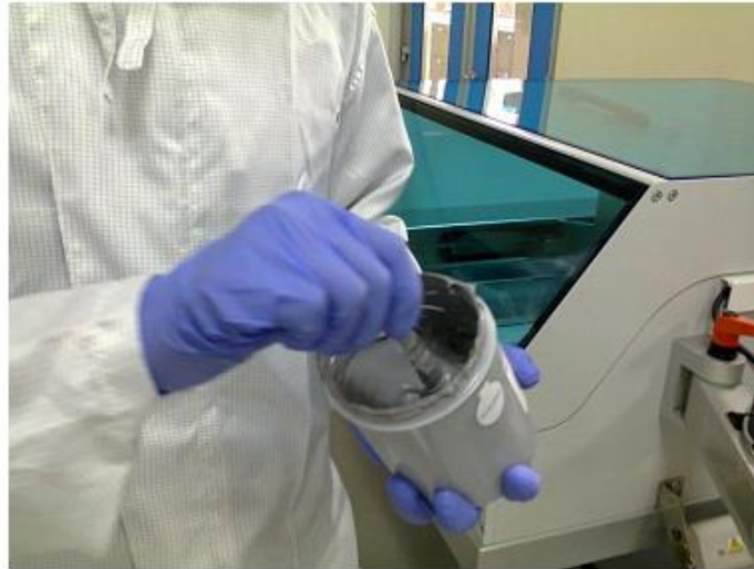
Figure12. Stirring of metal paste prior to printing
