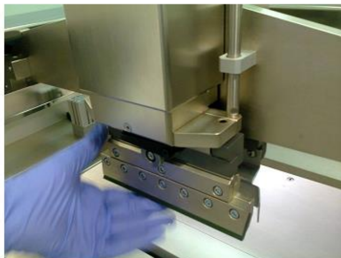
Figure 5. Front view of squeegee and scraper installed in the printing station
