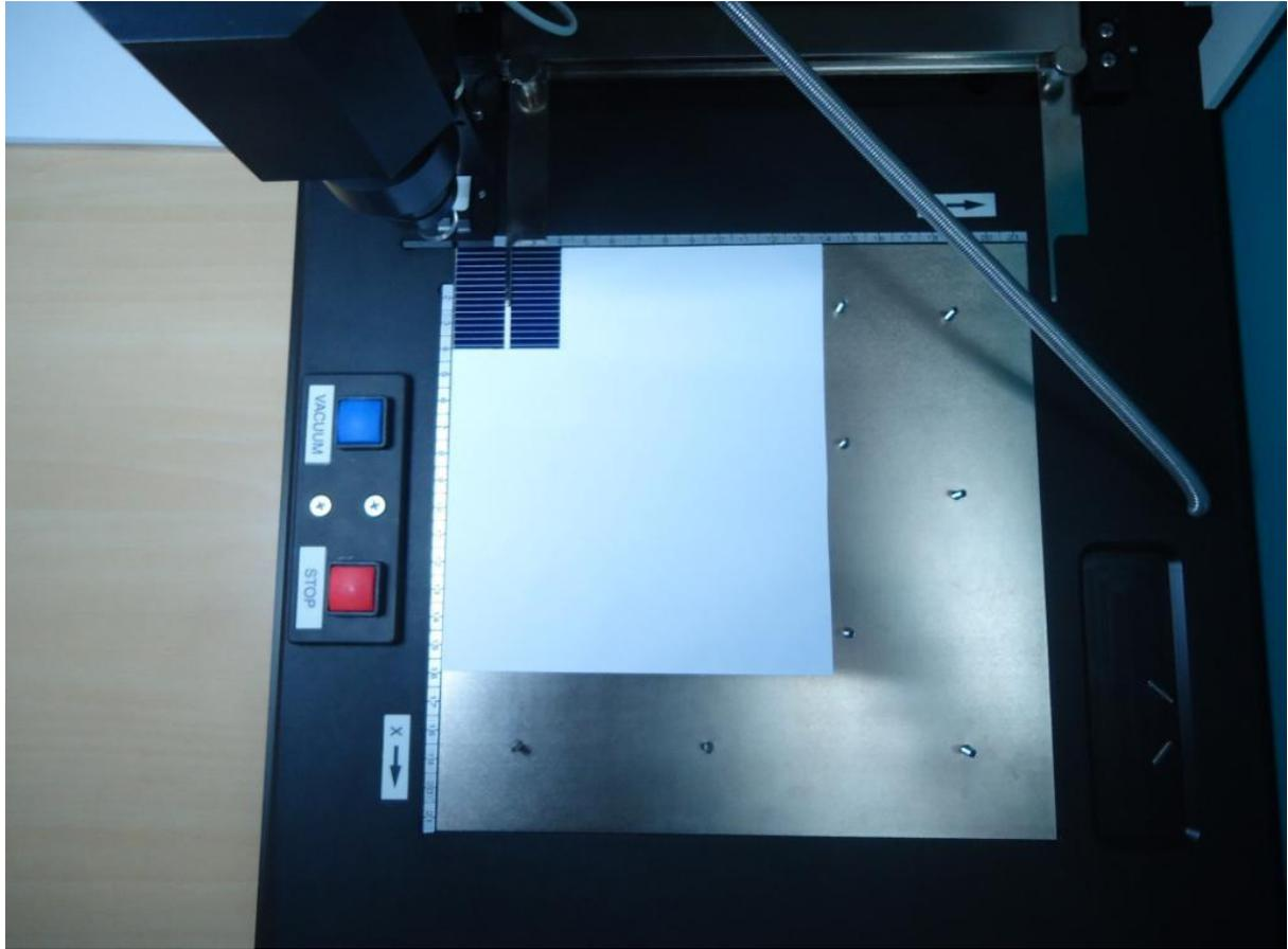
**Figure 5: Corescan system stage – Vacuum table and installed solar cell**
