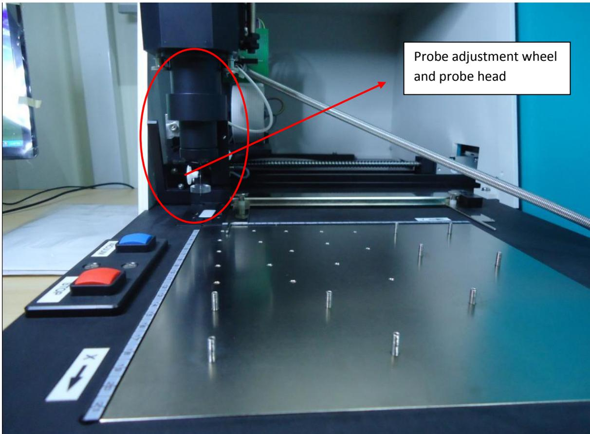
**Figure 4: Corescan system Stage**
