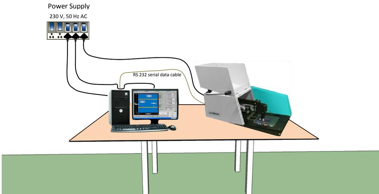
**Figure 2: Assembly of Corescan system**
