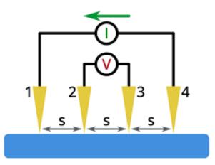
The required value of current is set through the sources. As current is passed through the two probes (say probe 1 and probe 4) a voltage respective to the current is produced in the other two probes (say probe 2 and probe 3). The voltage is measured through the voltmeter connected across the probes (say probe 2 and probe 3).
