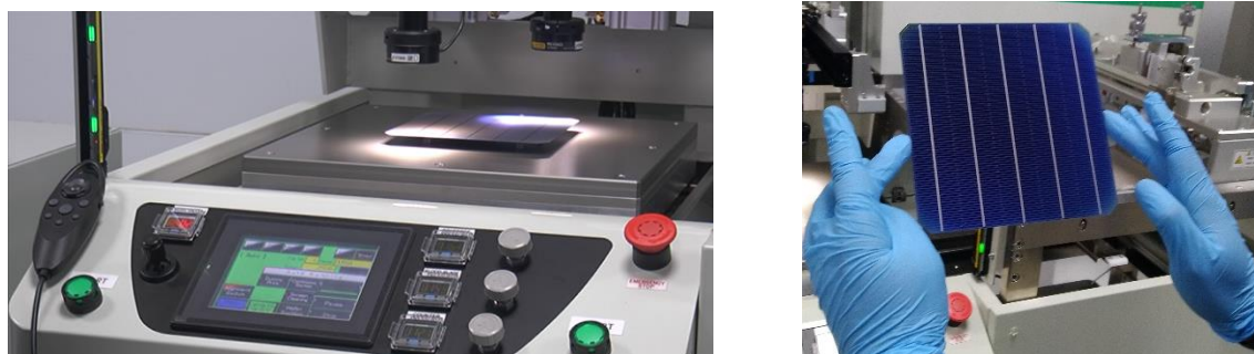
Fig.36:- Wafer lifting and handling after printing
