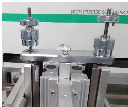
Fig.29:-Tightening the squeegee height adjustment
