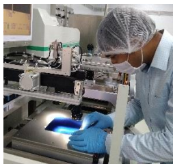
Fig.33:- Placing of Wafer on print table (a) Wafer area (b) wafer placed (c) Alignment mark.
