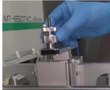
Fig.18: Flood plate height fixing
