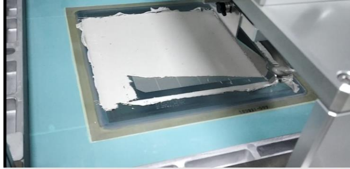
Fig.40:- Silver paste after flood stroke
