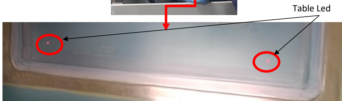
Fig.27: Screen alignment with Table LED light
