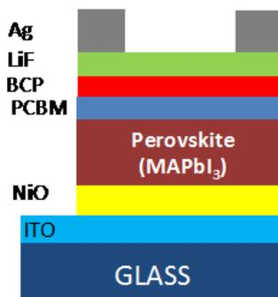
Fig.1 Schematic of semi-transparent perovskite device
