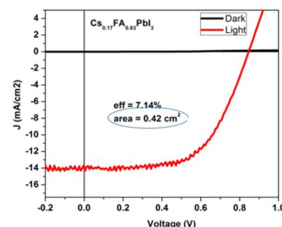
Fig. 3 J-V characteristics of mixed cation perovskite device under 1 Sun illumination
