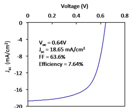
Fig. 2 J-V characteristics of semi-transparent perovskite device under 1 Sun illumination
