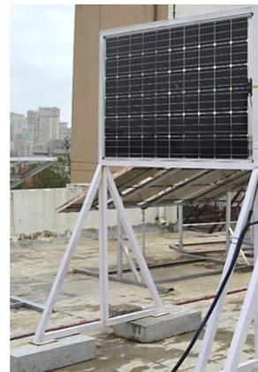
Vertically mounted bifacial solar panel, at NCPRE performance monitoring station at IIT Bombay, after 100 days of outdoor exposure. The panel was never cleaned!
