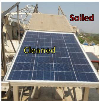
Two identical panels, mounted in the conventional way at the NCPRE PV performance monitoring station at IIT Bombay after 100 days of outdoor exposure. One is cleaned every day and the other is left to soil naturally.
