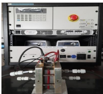
Redox flow battery test station (Fuel Cell Technologies Inc., USA) with single cell of 25 \text{ cm}^2 area
