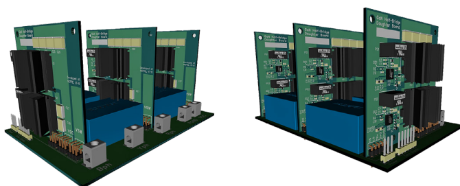
Figure: Power stage of driver with 3 daughter cards and DC-Link capacitors installed
