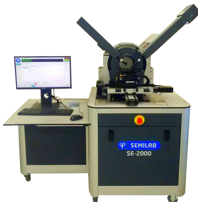
Figure : SE-2000 spectroscopic ellipsometer installed in NCPRE Si solar cell fabrication lab.
