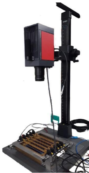
Fig: Lock-In-Thermography for silicon solar cells
