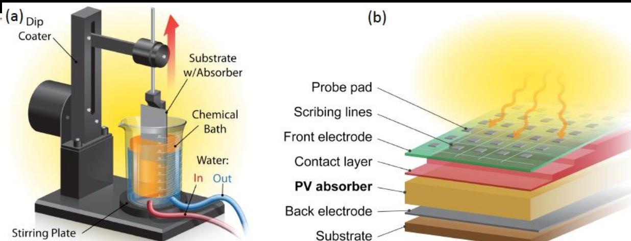
Schematic illustrations of (a) combinatorial dip-coating process for creating thickness steps in the CdS contact layer, and (b) PV device structure with integrated combinatorially deposited CdS contact layer/buffer layer
