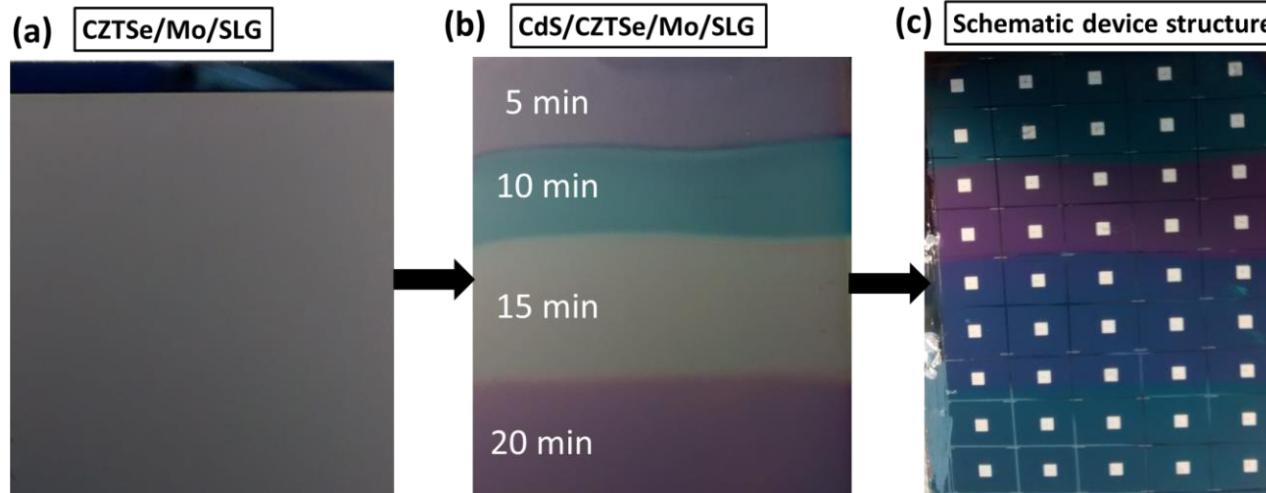
Fabrication stages of the combinatorial PV device library, after the deposition of (a) CZTSe absorber, (b) CdS contact with thickness steps, and (c) TCO and metal electrode pads
