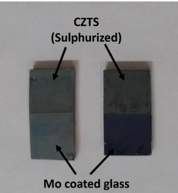
Annealing at 600°C, 15min in the presence of S in Ar atmosphere
