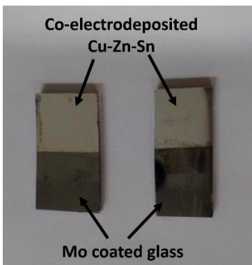
Electrodeposition at -1.15V for 20 min.
