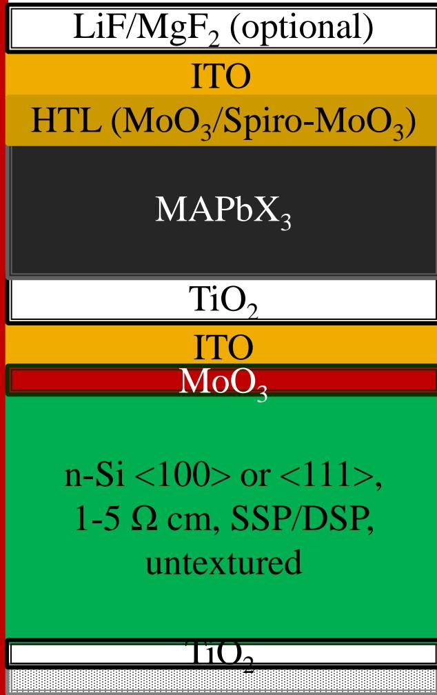
Bottom Cell: carrier selective contact (CSC) Si cell
