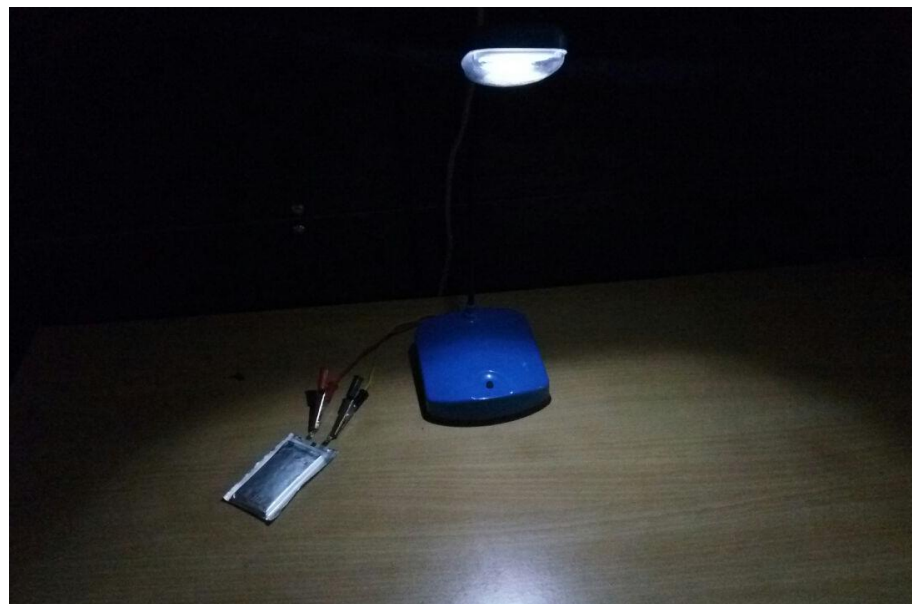
Study lamp powered by a pouch cell
